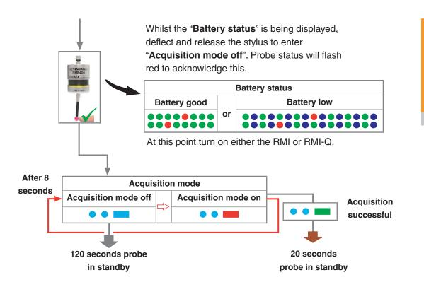
If partnering is unsuccessful "**Acquisition mode off**" will be displayed again after 8 seconds. Deflect the stylus for less than 4 seconds to select "**Acquisition mode on**" again.
