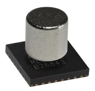
The AM4096Q is a rotary magnetic encoder IC which uses Hall sensor technology for sensing the magnetic field. It offers the same functionality as the AM4096 but comes in a small and compact QFN32 package (6 × 6 mm).
