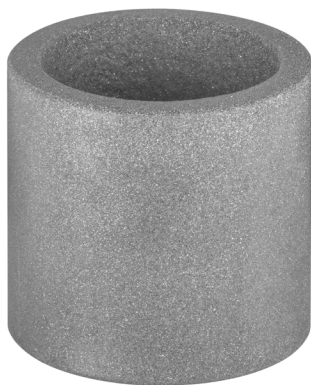
Silicon carbide test piece with a surface finish of 16 Ra
