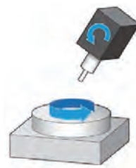
ISO 10791-6 reference = 'CK' CK: Head -Table machines Swivel head and/or rotary table
