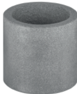
Figure 1 Silicon carbide test piece with a surface finish of 16 Ra.
