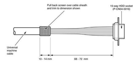
Preparation of Renishaw universal machine cable for shank mounted systems
