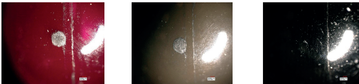
Figure 2 Microscope photos of the balls after the completed testing (1 – ruby ball, 2 – silicon nitride ball, 3 – OPTiMUM diamond coated).
