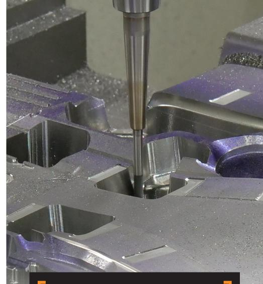
Standard Tool & Mold was experiencing some accuracy issues with smaller cutters, resulting in very small discrepancies between small diameter ballnose cutters. The original tool setting technique was not found to be repeatable, resulting in blending marks on critical surfaces.
