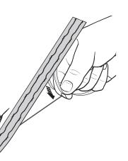
Engage the centre section removal tool and, with a consistent forward pressure, remove the centre section of the FASTRACK carrier.
