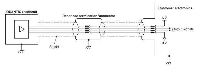
IMPORTANT: The shield should be connected to the machine earth (Field Ground). For JST variants the ferrule should be connected to the machine earth.
