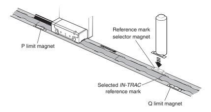
Apply firm finger pressure to the magnet via a clean, dry, lint-free cloth to ensure complete adhesion
