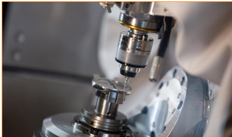
RMP24-micro probe inspecting a watch component
