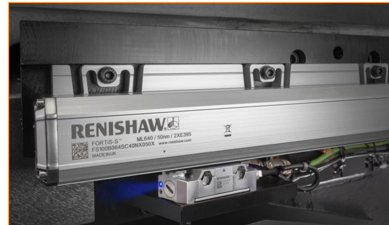
FORTiS encoder installed on a machine tool
