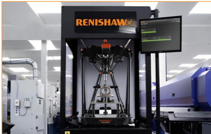
Equator gauge inspecting parts on the shop-floor
