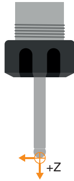
2 Manually set a nominal tool frame where +Z points out of the artefact
