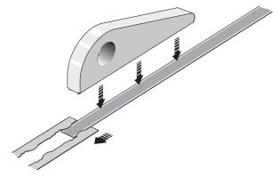
2. Place thumb and forefinger either side of the through hole and push/pull the scale through the FASTRACK carrier.
