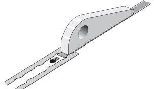
Feed the scale through to the end of the FASTRACK carrier or into the optional end-cap (if used).
