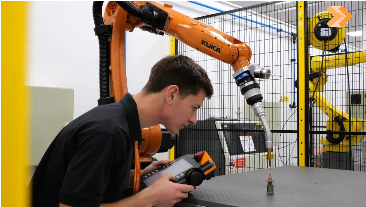
Legacy pin-to-pin robot commissioning
