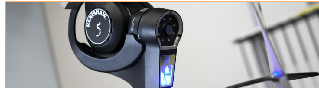
RFP1 measuring an aerospace blade
