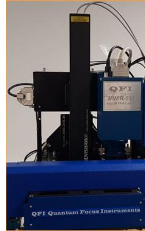
Virsa attached to a QFI semiconductor thermography system
